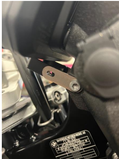
*NOTE - the position of the lower mounting extension brackets. The slot should be rearward. This gives you some adjustment if required, to get a perfect gap all the way around between the display and the brace as shown on step 8.
